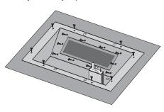
11) Carefully lift the burner tray assembly out. Be careful not to tear gaskets when lifting out the valve tray; these gaskets seal the valve from the exterior of the firebox.
